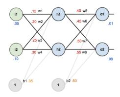
The blue numbers are the training inputs/outputs, the red numbers are the weights and the orange numbers the biases. Calculate the forward passes and backward passes from Algorithm 33 in the lecture and update the weights.
